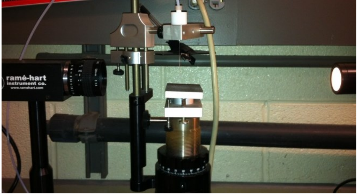
Figure 4.1. Ramé Hart goniometer used for droplet evaporation rate and surface tension measurements: camera on left, needle for droplet suspension in middle, and backlight on right. Repeated with permission from [51].
