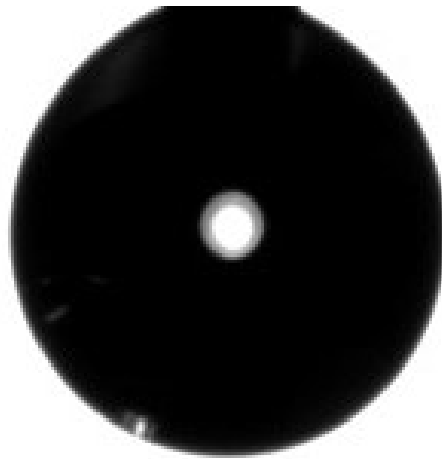
Figure 4.2. An image captured by the goniometer and used for determination of drop geometry and surface tension.
